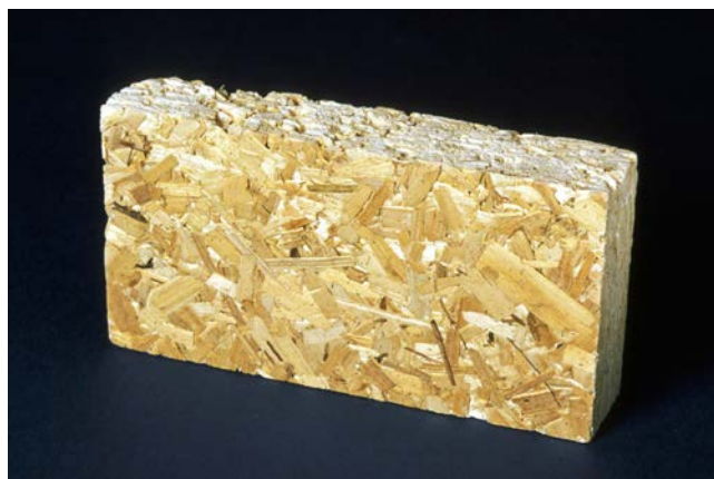
Fig. 22. Experimental fiberboard made with hemp. (Courtesy Dr. K. Domier, Univ. Alberta, Edmonton.)
